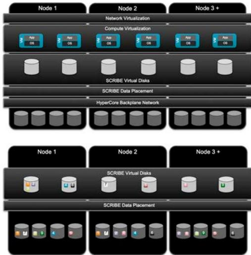
We did ask Scale Computing about using erasure coding or different RAID schemes for data protection, and they said that they felt that they would rather have their CPUs servicing VMs than dealing with the added complexity. Furthermore, cheap storage made the marginal benefits of storage efficiency moot.
